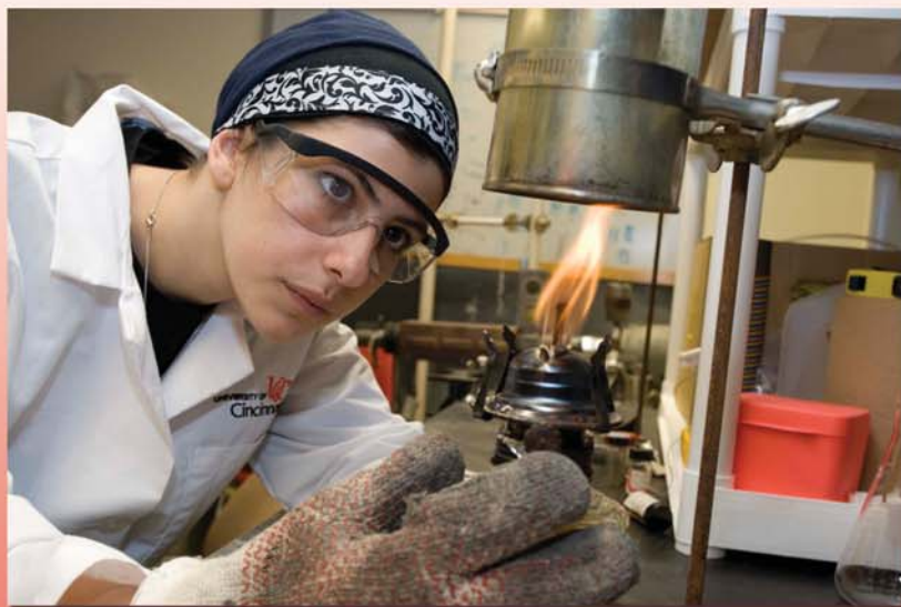
Maesa Idries, a Chemical and Materials Engineering major, experimenting to quantify nano-particles in Diesel engine exhaust using small angle x-ray scattering. Mentor: Dr. Greg Beaucauge
