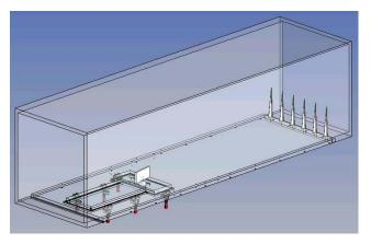
Experiments are performed in a subsonic wind tunnel with a special test section that is used to study unsteady flow separation behind generic protrusions to simulate flight conditions of an airplane with appendages installed on the fuselage (cameras, antennas, probes, etc). The experiments enable research of the correlation between the flow field, unsteady pressure, and vibrational modes induced on a fuselage panel.
