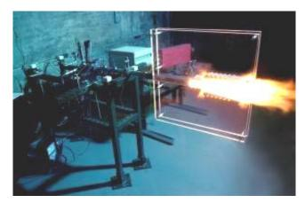
A pulse detonation engine (PDE) offers few moving parts, high efficiency, high thrust, low weight, low cost, and ease of scaling. These make the PDE an attractive alternative to jet turbine engines for small disposable engines. The near constant volume heat addition process, along with the lack of a compression cycle, lend to the high efficiency and specific impulse, simplicity, and lowcost of pulse detonation engines.
