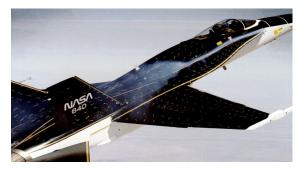
Lift force on delta wings at a high angle of attack relies on large-scale vortices that separate at the leading edges of the wing. At high angle of attack these vortices loose gradually their coherence due to intrinsic flow instabilities that lead to vortex breakdown. At these conditions, the lift produced by the vortices is reduced causing loss of controllability and stall.
